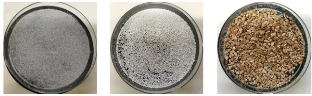
Micro-porous Silica gel Composite SG / 30 wt.% LiCl Composite Verm / 45 wt.% LiCl
