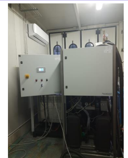
Large-scale (90 kW-HT) and low-scale (35 kW-HT) prototypes testing rigs
